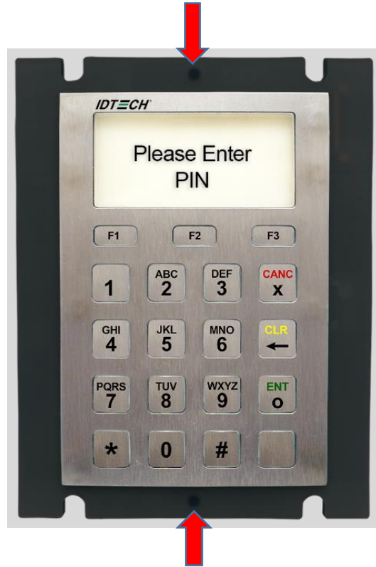
Tamper-detection buttons are at the top and bottom of the front face.
